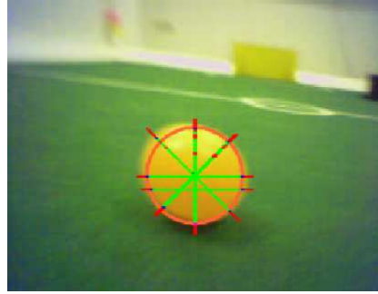
Figure 2.3: Ball percept with scan lines. (Röfer et al., 2004, Fig. 3.10a)
