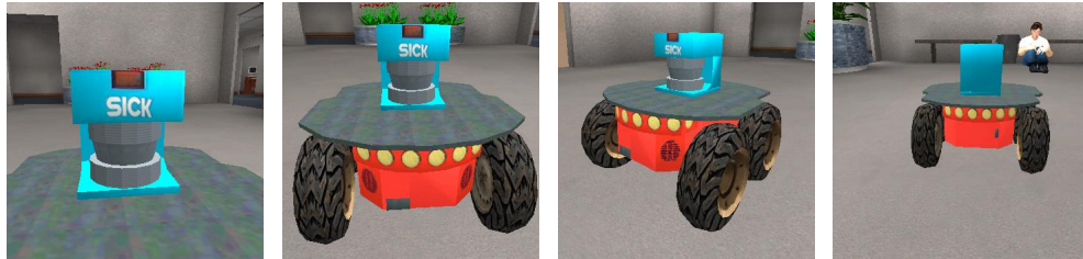
Figure 6.7: Sensors. The SICK laser range scanner on top and the front and back sonar rings are clearly visible. The other sensors like the VictimRFID sensor and INU sensor are hidden or attached to the bottom of the robot's chassis.
