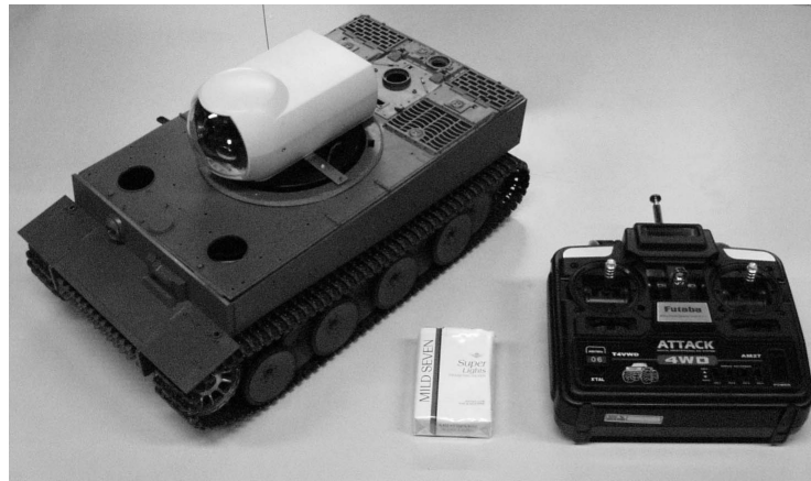
Fig. 2. Picture of the robot : CCD camera on the main body
