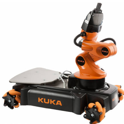
Figure 1: A KUKA youBot on four omnidirectional wheels with a single 5 DoF arm
