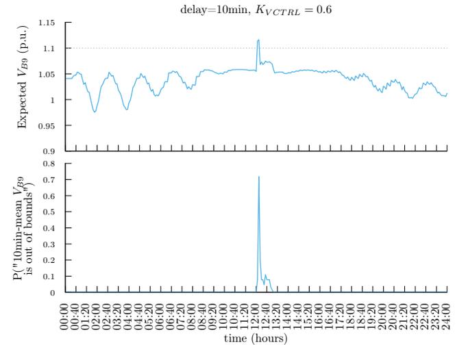
Fig. 7. Expected  $V_{B9}$  voltage profile and probability that  $V_{B9}$  goes out of bounds at different time, for  $K_{VCTRL} = 0.6$ , when control delay is 10 min.
