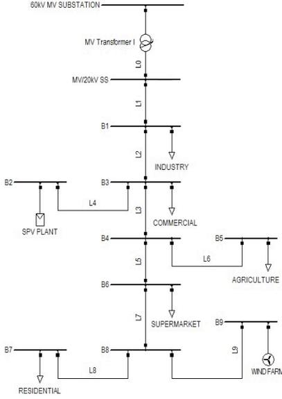
Fig. 1. Diagram of MV smart grid from SmartC2Net.
