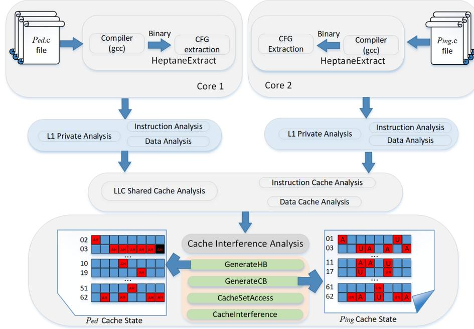
Fig. 3. The architecture of the Cache Interference Framework
