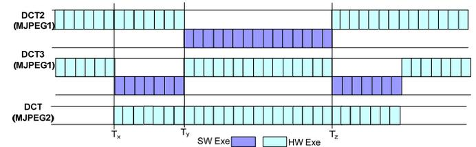
Fig. 3. DCT Execution snapshot in MJPEG1/MJPEG2 (AMAP)
