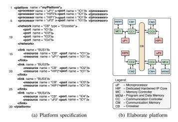
Fig. 4. Example of a Daedalus MPSoC platform.
