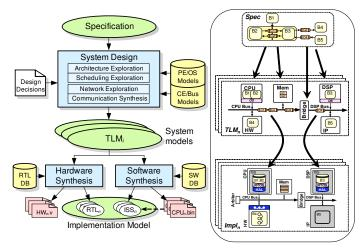
Fig. 5. System-On-Chip Environment (SCE) design flow.
