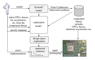
Fig. 7. ESL design flow using SystemCoDesigner.
