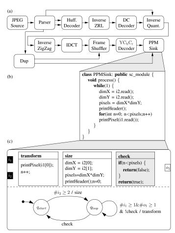
Fig. 8. Block diagram of a Motion-JPEG decoder. b) shows the SystemC code of an actor that can be transformed into a SysteMoC actor given in c).
