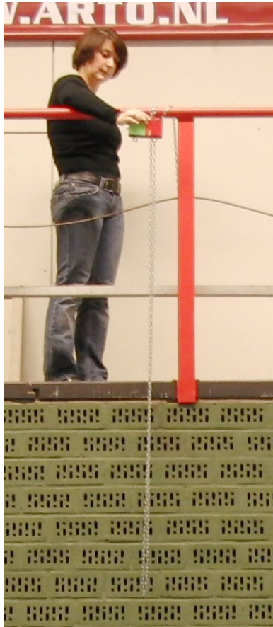
Figure 4. Dropping two wooden blocks simultaneously from a height of a few metres, while one of the blocks is chained and the other is in free fall.
