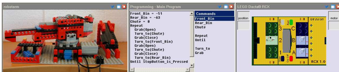
Figure 2. A computer microworld for manipulating a robot arm.
