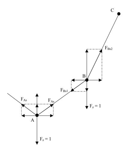
The (equal) weights lead to a gravitational force  $F_z$  in each point of application. For simplicity we take  $F_z = 1$ .
