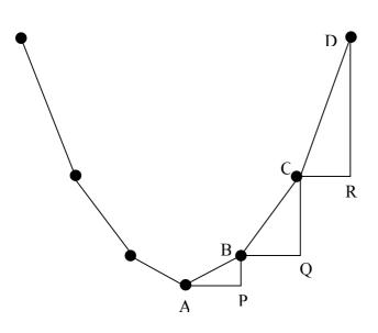
The videoclip shows a chain on which hang five equal weights. These weights have placed symmetrically such that the horizontal distance is always 1 dm. Coordinate system and scaling have already been chosen.
