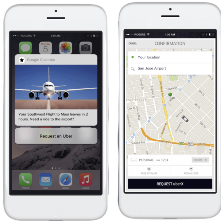
Figure 3: Illustration of the case of custom redirect URIs - when the user clicks on a link and instead of opening the browser window it opens the app.
