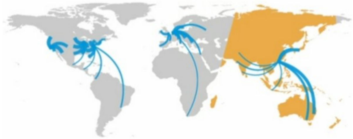
Figure 3.4: Anycast routing - Routing client traffic to the nearest data center location all over the world.
