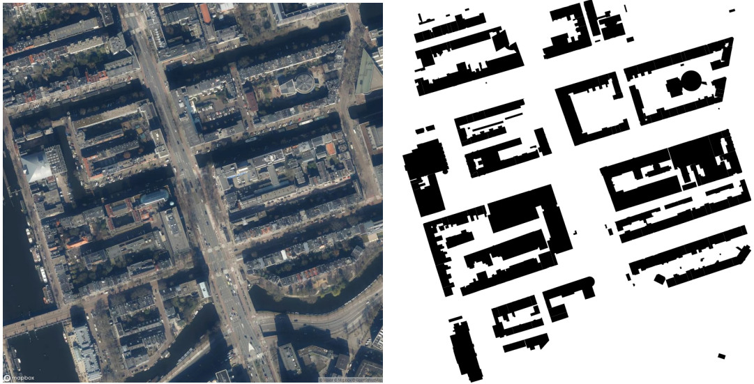
Figure 4.3: Sample of satellite view image ( left ) and 2D projection slice at a targeted height of 8 metres above the terrain ( right ) obtained at the completion of the pipeline.
