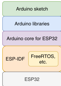
Fig. 1: Simplified view of the software stack for Arduino code execution on ESP32. The original FreeRTOS, also referred to as vanilla FreeRTOS, is a single-core RTOS. To support dual-core ESP targets (like our board), it has been modified and integrated into ESP-IDF (Espressif IoT Development Framework) [20], forming what is known as IDF FreeRTOS [21] or ESP-IDF FreeRTOS [22]. In order to use it through the Arduino IDE with Arduino libraries, we rely on a compatibility layer [23], the Arduino core for ESP32.
