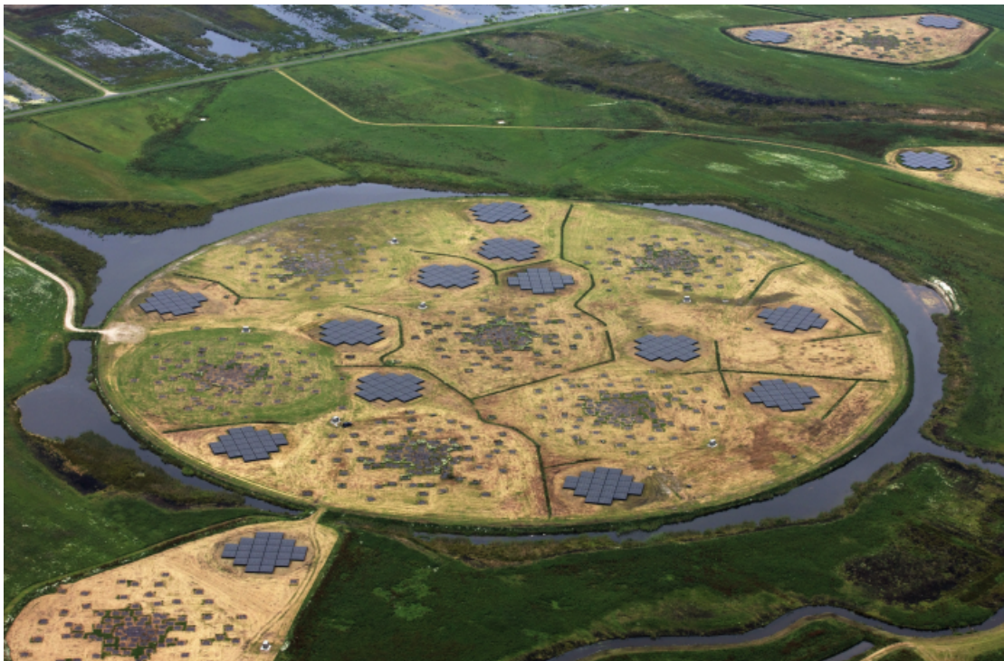
Figure 2.2: A 2011 aerial photograph of the Superterp, the heart of the LOFAR core. Six core stations can be seen in the circular island, with three additional LOFAR stations in three smaller islands in the lower-left and upper-right corners of the photo(2)
