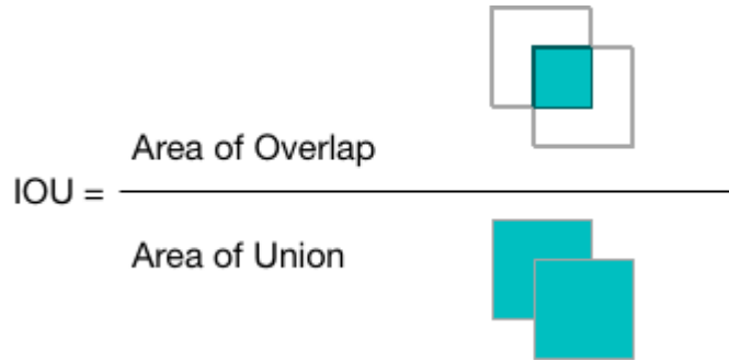
Figure 6.2: Computing the Intersection of Union is a division of the area of overlap between the bounding boxes by the area of union
