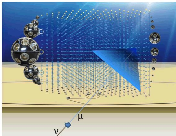
**Figure 1.1:** Artist's impression of the KM3NeT neutrino telescope placed in the depth of the sea. The figure explains how the DOM spheres are distributed in a cubic shaped area. Also, the conical beam of Cherenkov light was depicted as an effect of neutrino interaction with matter in the Earth. (source: [www.km3net.org](http://www.km3net.org))
