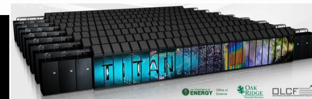
A few scientists run their computations on big machines. (like this 560640 core, 17 PFlop/s Titan at Oak Ridge National Laboratory)
