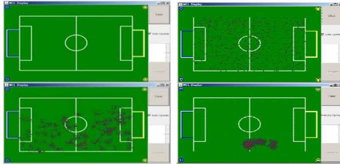
Fig.4. Estimating Process Using Particle Filter
