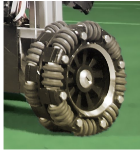
Fig. 1. Omniwheel designed and built by CARPE NOCTEM
