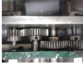
**Fig. 25** First reduction stage with spur gears.
