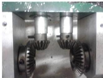
**Fig. 26** Second stage of reduction with bevel gears.
