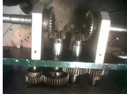
**Fig. 27** Final transmission system with the two stages.
