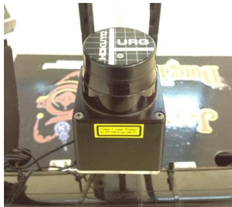
Fig. 8. A 2D laser range finder at the robot base for localization and mapping
