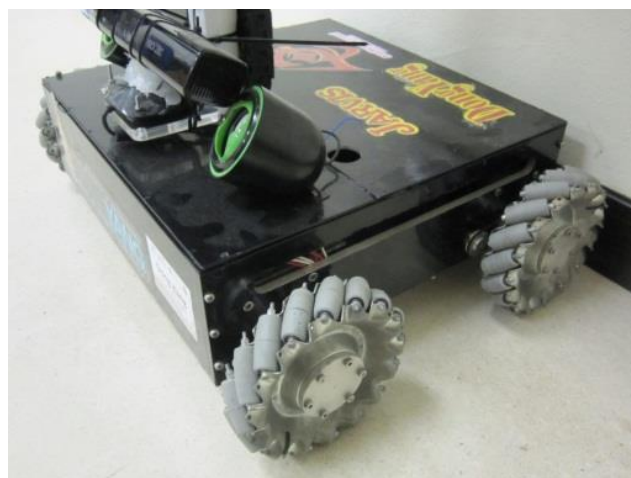
Fig. 4. The robot base with 4-Mecanum wheels
