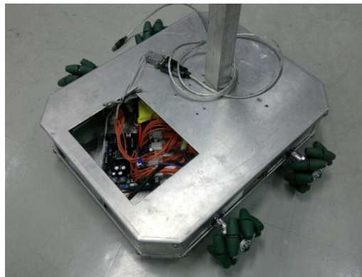
Figure 6. prototype mecanum robot.
