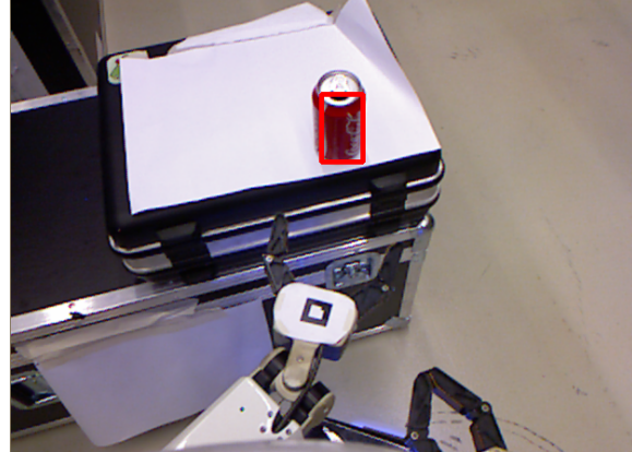
Fig. 5. Camera view with the gripper with ar-marker as well as object to grasp in sight.
