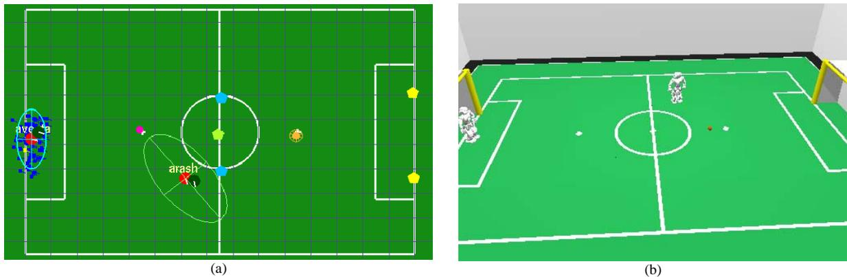
Fig 3. (a) Goalie's world model with a wrong symmetrized player position. b) Agents' real location in the *SimRobot*
