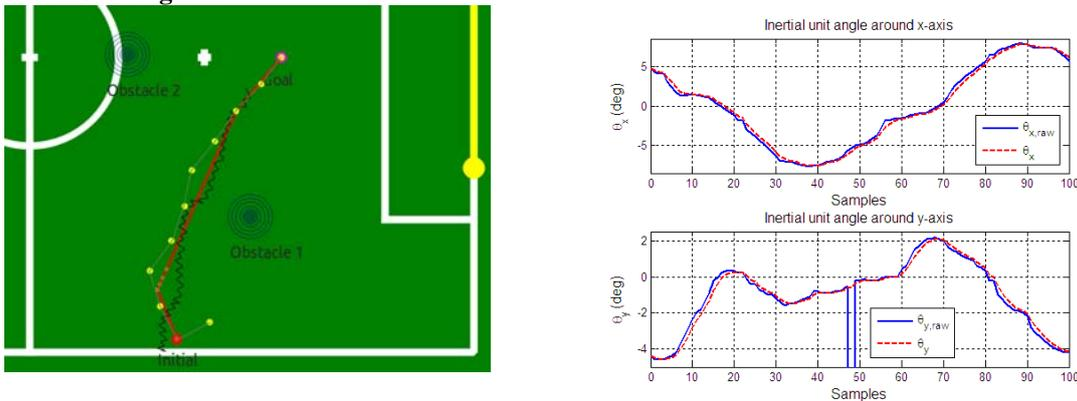
Fig A1. (a) Robot's experimental data on the RRT smoothed path; (b) filtered data of the inertial units for the walk engine
