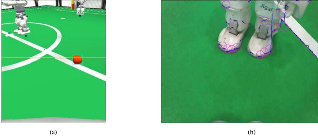
Fig 1. (a) ; Landmark and robot detection with simultaneous images captured by both cameras; (b) Robot detection
