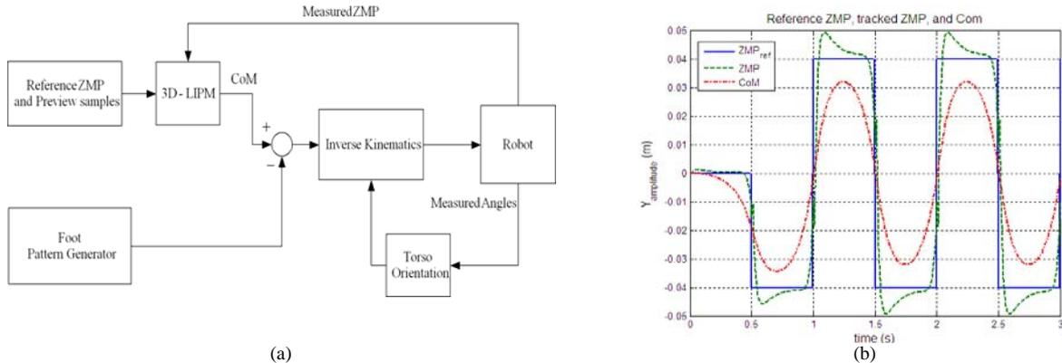
Fig 6. (a) MRL SPL walk engine and controller diagram; (b) ZMP and CoM position estimation
