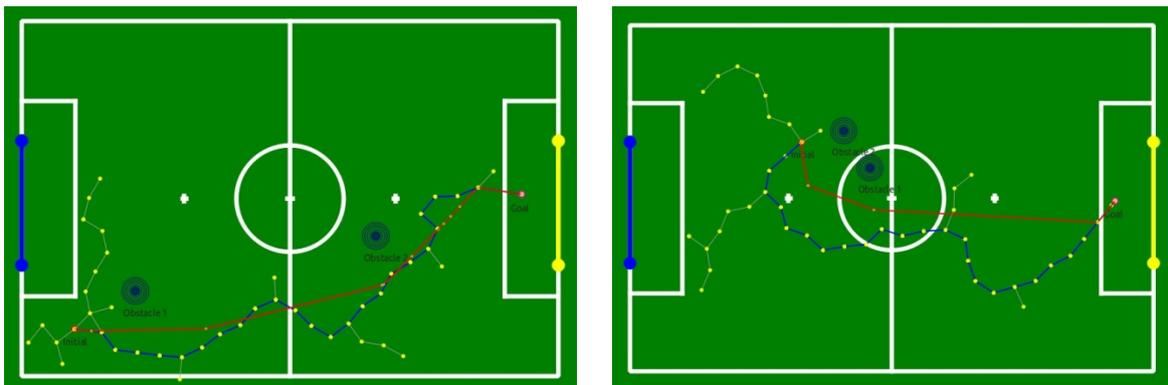
Fig 4. RRT generated and smoothed paths for two different maneuvers with obstacle avoidance
