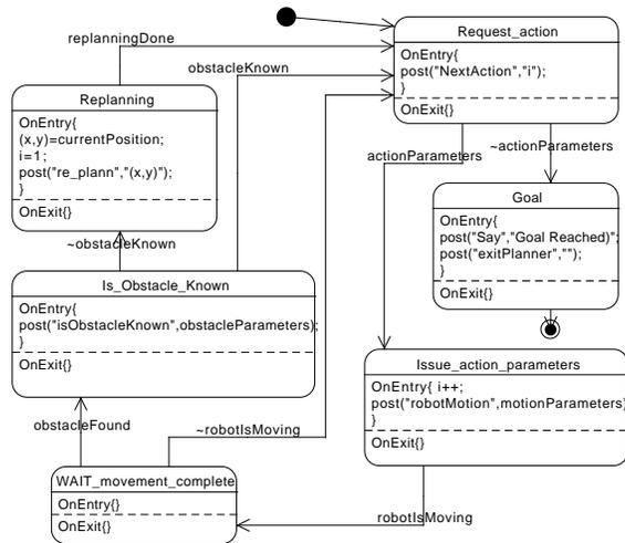
Fig. 6: The LLFSMs interpreted (and also compiled) used to run the plan, execute, re-plan cycle in our experiments.
