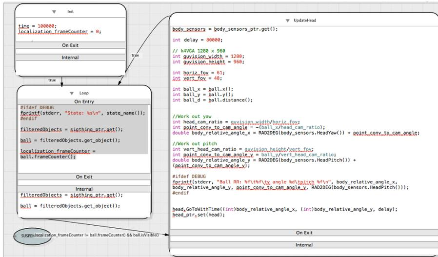
Fig. 1: A two-state LLFSM that implements a reactive control to track the ball.
