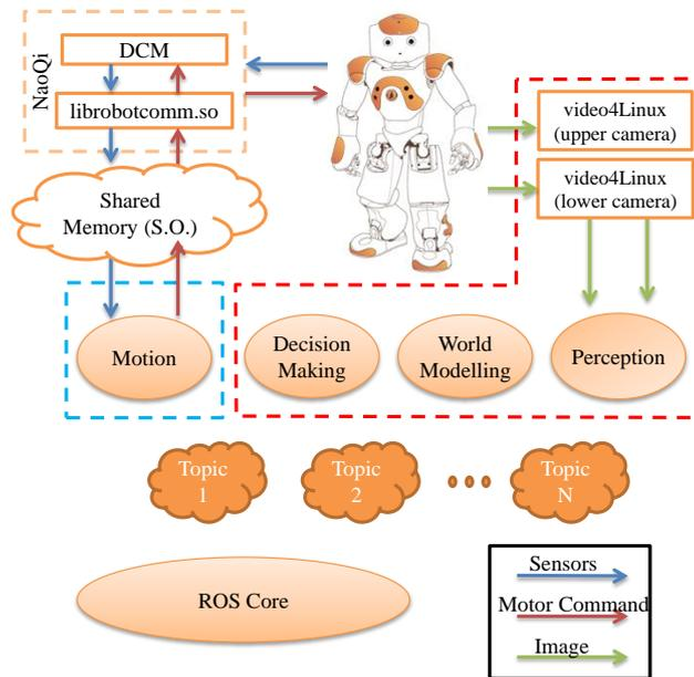
Fig. 1. Block Scheme of Our New Core with ROS
