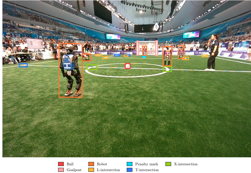
Fig. 3: Example of fully annotated image from dataset, taken at the World Humanoid Robot Games 2025 in Beijing (RCAP Beijing Masters 2025).
