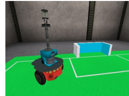
(b) A simulated P2DX robot mounted with a catadioptric omnidirectional camera and a SICK laser range sensor.
