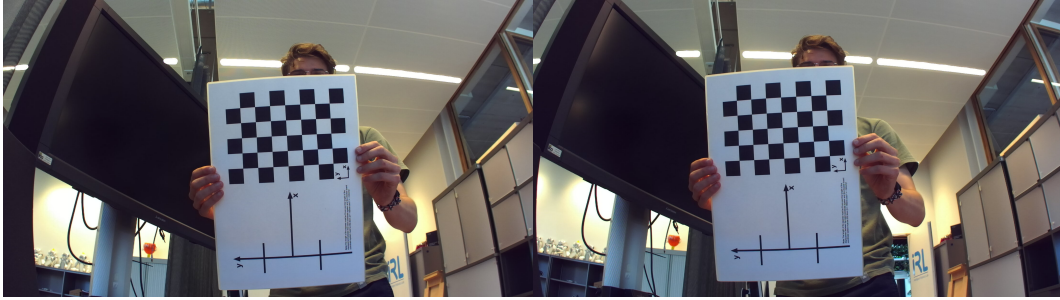
Figure 3.7: One of the views of the chessboard used to calibrate the ZED M device
