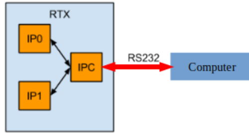
Figure 2.4: Communication between the arm and the computer
