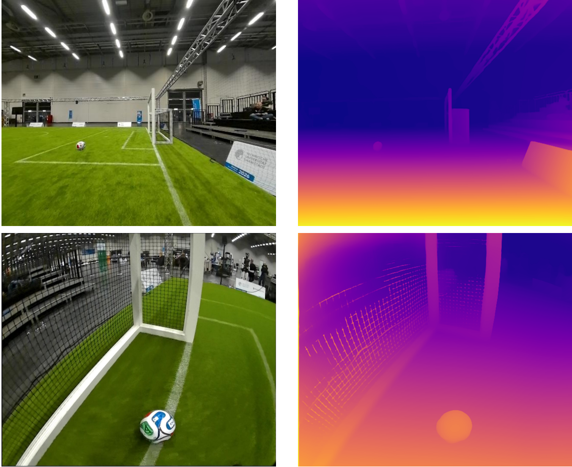
Figure 4.2: Two high-quality image pairs from the HSL Objects V1 dataset, with depth maps generated by DepthAnythingV2-Large.
