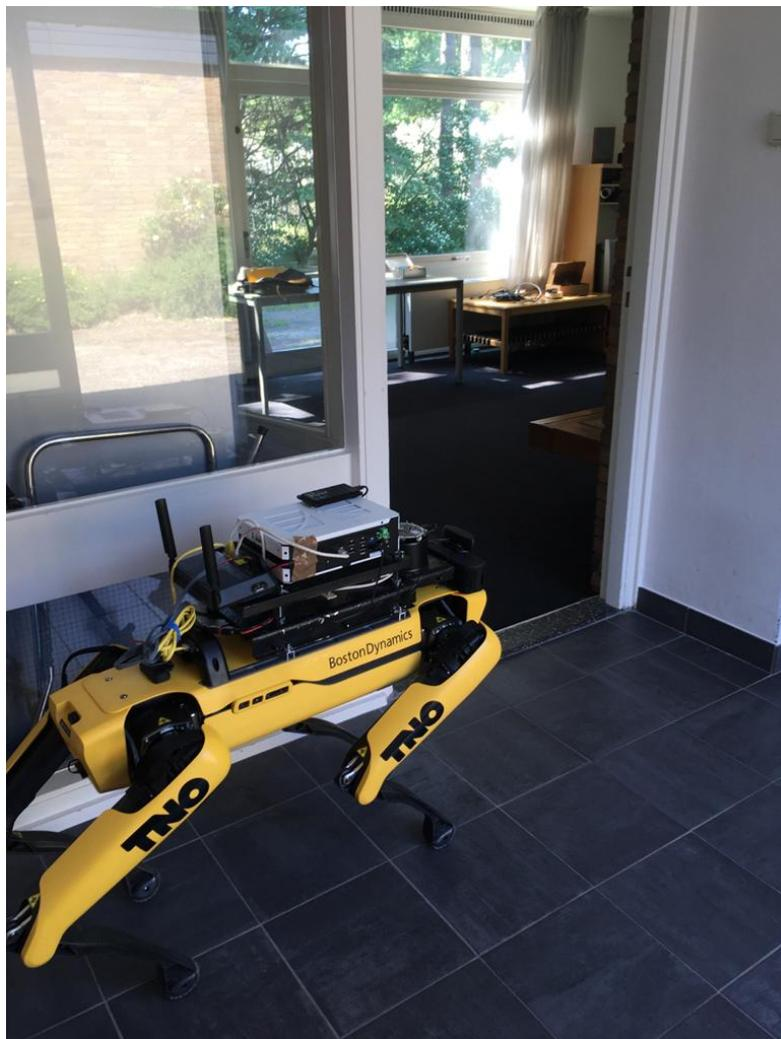
Figure B.1: Pose of the SPOT robot when capturing the point cloud shown in Figure 8.4c. Note the vertical line that is visible through the window, which was detected by the SPOT robot as door jamb (false positive), since the point cloud did not capture the left door jamb correctly.
