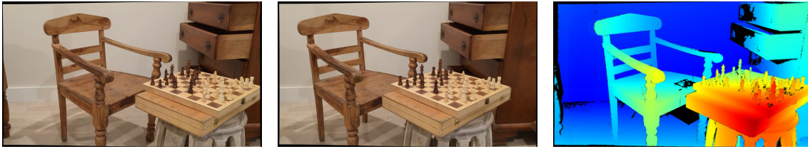
Figure 4: Disparity map (right) obtained with a mobile device on a robot arm, using the technique of [7]
