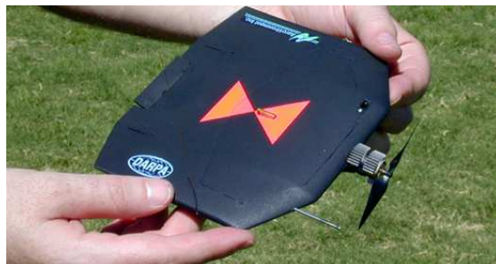
Figure 1: The Black Widow [Grasmeyer et al., 2001] was the first operating micro aerial vehicle system, a development which was finalized in 1999 by AeroVironment for Defense Advanced Research Projects Agency (DARPA). The Black Widow can fly for up to 20 minutes and carries a very small color video camera.
