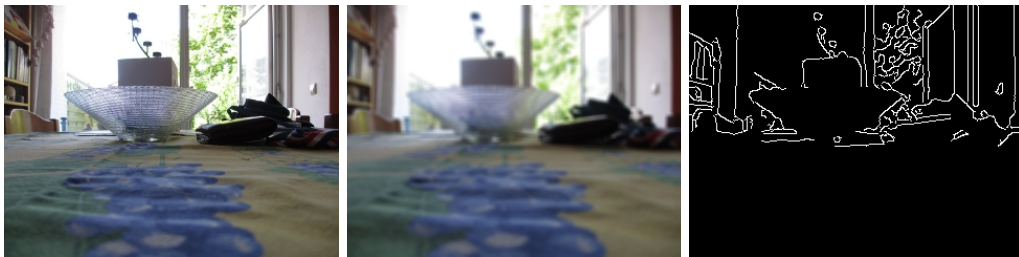
Figure 5: Left: Original image. Middle: Smoothed image. Right: Canny Edge Detector
