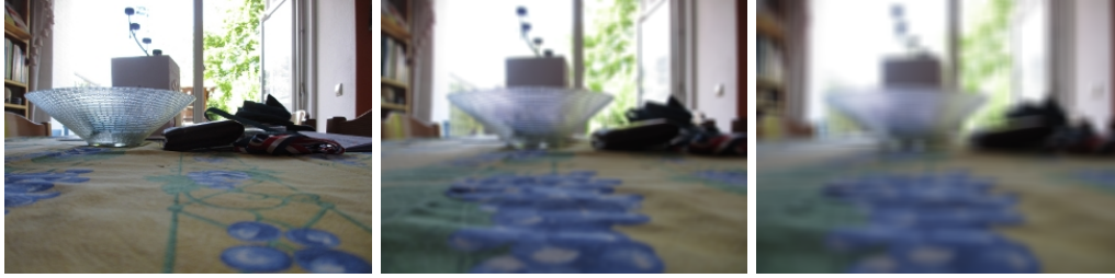
Figure 13: Left: original. Middle and right: Gaussian Blur of 3 and 11 pixels.
