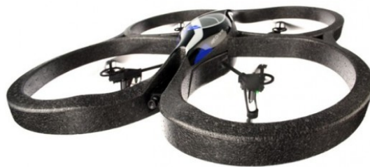
Figure 2: The Parrot AR.Drone is equipped with two cameras and several inertial sensors. The development is driven by commercial and research purposes. The small quadrotor allows remote observation of hazardous environments inaccessible for humans and ground robots.
