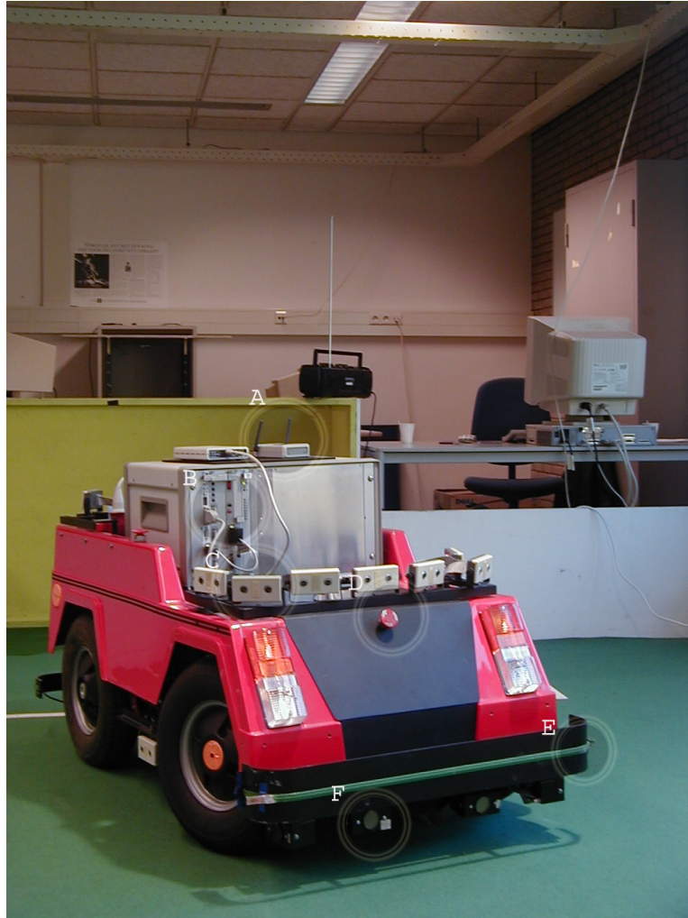
Figuur 3.4: MARIE A:breezenet wireless netwerk B: computer C: Robosoft ultrasoon sensoren D: stop knop E: bumper sensor F: Polaroid ultrasoon sensoren
