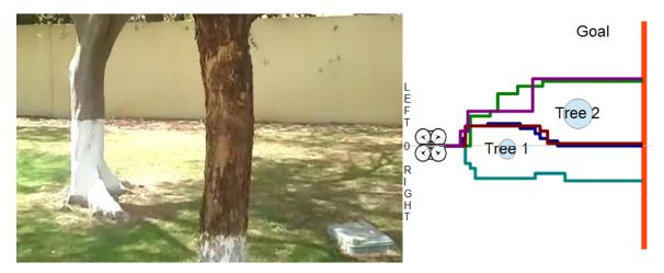
Figure 5.13: (Left) Frame consisting two trees as obstacles (Right) Drone flight path avoiding the trees in 5 successful runs using the proposed method
