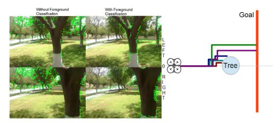
Figure 5.10: Drone flight frames illustrating results of the proposed method without Background/Foreground Classification (left) and with Background/Foreground Classification (middle) and flight results (right) avoiding 1 obstacle
