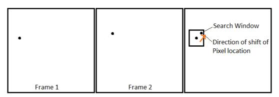
Figure 3.4: Illustration of Optical Flow of a moving pixel in consecutive images
