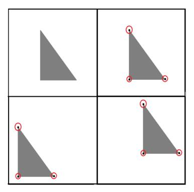
Figure 3.2: (Top-Left) a simple Grayscale image of a triangle. (Top-Right) the same image with best rated corners found by the Harris Corner detector. (Bottom-Left and Right) same corners found despite location of triangle in image.
