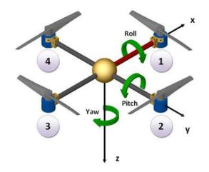
Figure 5.3: illustration of pitch, yaw and roll on quad-rotors
