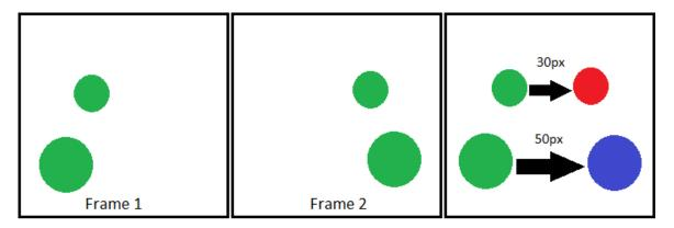
Figure 3.6: Illustration of two balls rolling from left to right in Frames 1 and 2. The right frame shows the shift in pixels from Frame 1 to Frame 2 and segments them based on distance moved where the Blue ball is considered closer and the red ball considered further away from the camera.
