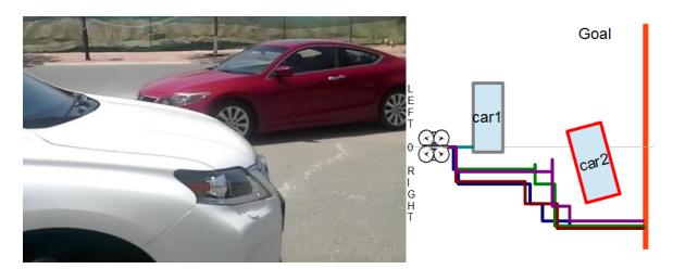
Figure 5.17: (Left) Frame consisting of two cars as wide obstacles. (Right) Drone flight path avoiding the trees in 4 successful runs and 1 failed run (turquoise) using the proposed method
