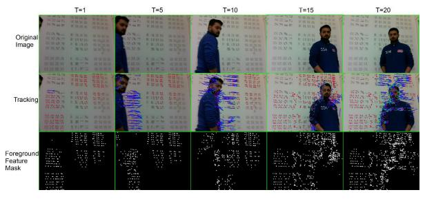
Figure 5.6: Results tracking step without using the proposed background subtraction step. (Top row) original images, (middle row) tracking using Lucas-Kanade pyramid optical flow algorithm and (bottom row) foreground feature mask generated after tracking, clustering and segmentation
