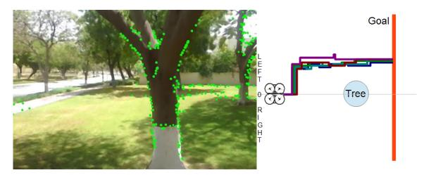
Figure 5.11: Drone Flight avoiding the tree in 5 successful runs without using depth segmentation or proximity estimation (algorithm 3)
