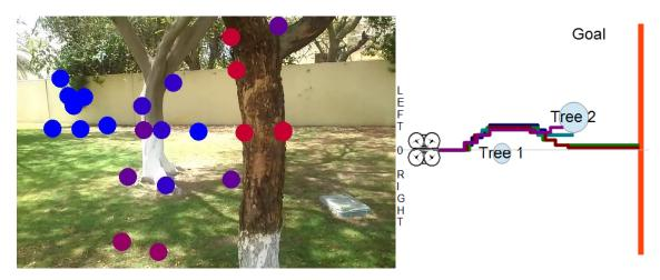
Figure 5.16: Drone Flight avoiding the trees in 2 successful runs using only proximity estimation
