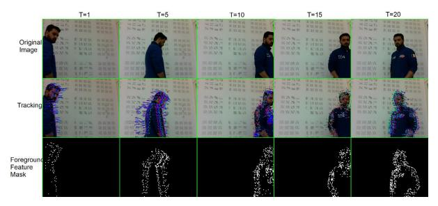
Figure 5.5: Results from the proposed method of tracking motion input from the background subtraction module previously and clustering feature points. (Top row) original images, (middle row) tracking using Lucas-Kanade pyramid optical flow algorithm and (bottom row) foreground feature mask generated after tracking, clustering and segmentation
