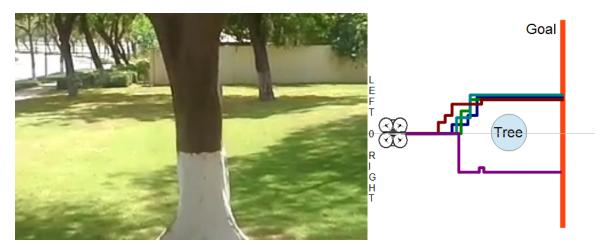
Figure 5.9: (Left) Frame consisting single tree as an obstacle. (Right) Drone flight path avoiding the tree in 5 successful runs using the proposed method
