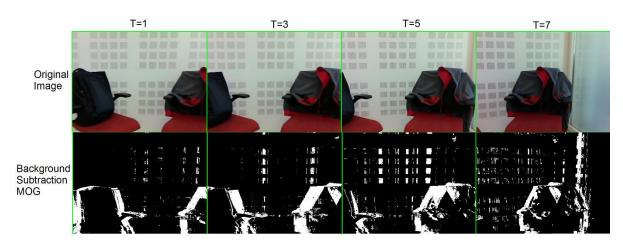
Figure 4.2: Foreground mask generated from Background Subtraction using Mixture of Gaussians with the camera direction moving left to right in a fixed scene
