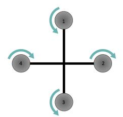
*Figure 5.2: Skeleton of a quad-rotor illustrating direction of rotation of each of the four rotors.*
