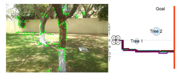
Figure 5.15: Drone Flight avoiding the trees in 5 successful runs using only optical flow
