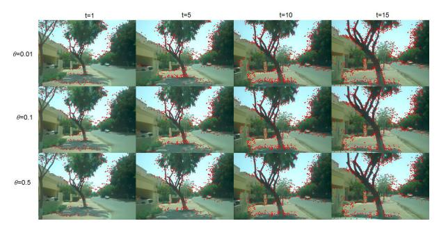
Figure 4.5: Comparison of feature detection results at different corner score thresholds  $\theta$  for an outdoor scene
