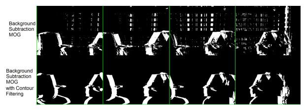
Figure 4.3: Results of Background Subtraction using Mixture of Gaussians with and without contour filtering
