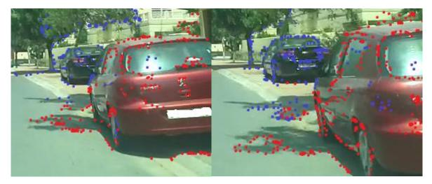
Figure 4.8: Results of Depth estimation in a moving scene from Optical Flow. (Left) Frame at t=10. (Right) frame at t=14. Red dots denote features moving at a faster rate and Blue dots denote slower moving features
