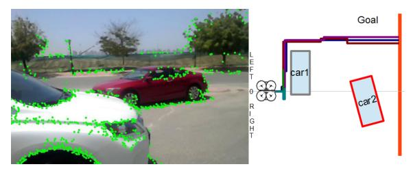
Figure 5.19: Drone flight results with 3 successful runs and 2 failed runs (green and turquoise) using only optical flow
