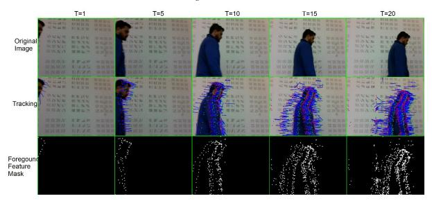
Figure 5.7: Results from the proposed method of tracking motion input from the background subtraction module previously and without clustering feature points. (Top row) original images, (middle row) tracking using Lucas-Kanade pyramid optical flow algorithm and (bottom row) foreground feature mask generated without clustering
