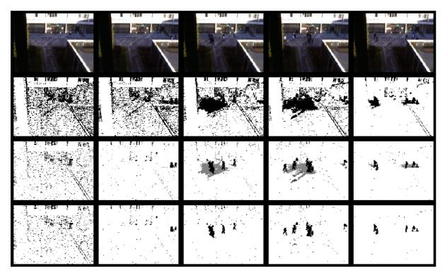
Figure 3.1: The top row consists of the original frame sequence at frames 15, 105, 235, 290 and 1200 respectively. The second row shows the results from Grimson et al's. The last two rows are the result of the method proposed by Bowden et al where the white pixels are the background mask and the foreground is the black pixel regions without and with shadow removal. Courtesy [4].
