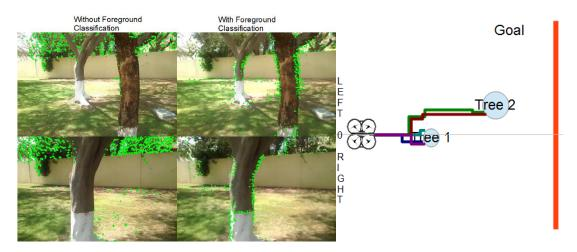
Figure 5.14: Drone flight frames illustrating results of the proposed method without Background/Foreground Classification (left) and with Background/Foreground Classification (middle) and flight results (right) avoiding 2 obstacles
