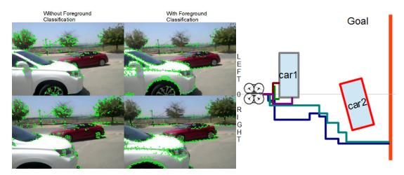
Figure 5.18: Drone flight frames illustrating results of the proposed method without Background/Foreground Classification (left) and with Background/Foreground Classification (middle) and flight results (right) avoiding 2 wide body obstacles
