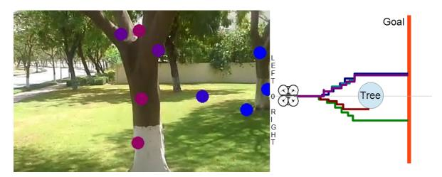
Figure 5.12: Drone Flight avoiding the tree in 4 successful runs using proximity estimation
