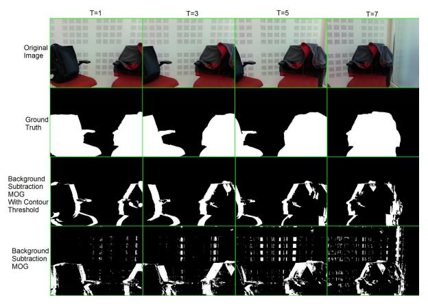
Figure 5.4: Results of the proposed extension on the standard OpenCV implementation of background subtraction using MOG
