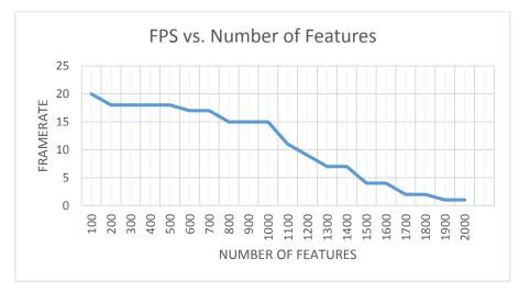
Figure 5.8: Graph of system performance with respect to frame-rate (FPS) against number of features detected
