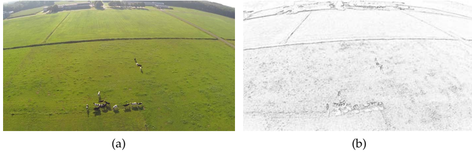
Figure 9: (a) The original image. (b) The gradient magnitude energy image, I_e . We find that the edges found in the original image become visible.
