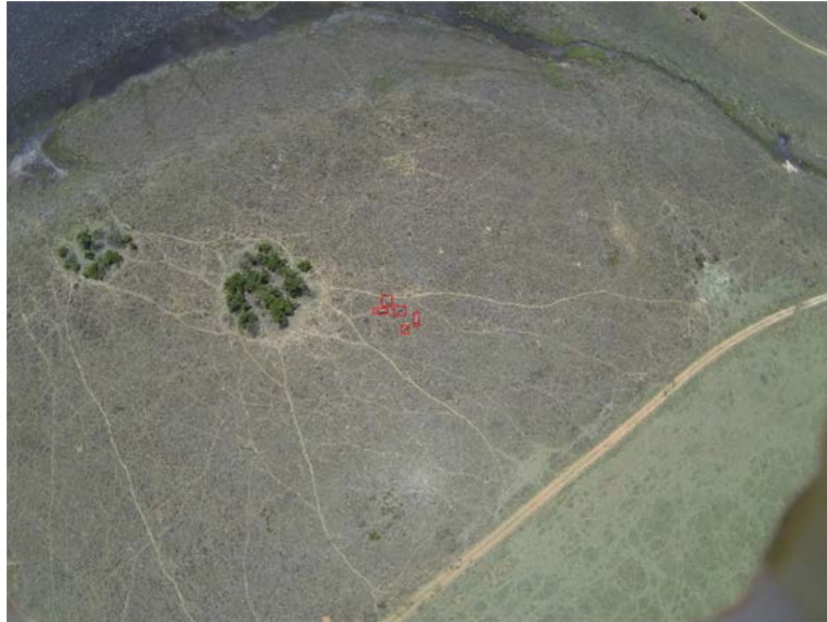
Figure 2: Example output of an automatic object detection algorithm on an image taken from the RHINOS dataset.
