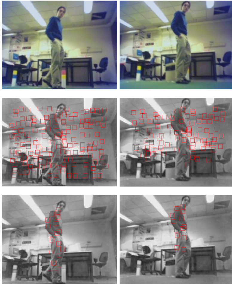
Figure 2.7: Tracking 150 features using the KLT algorithm. Top: the original images. Middle: all features selected in the first image and the remaining ones after tracking (63%). Bottom: manual selection of features on person. 70% of them are tracked, all correctly.
