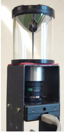
Figure 3.1: IAS Group Omnidirectional Camera, consisting of a Dragonfly<sup>®</sup>2 camera and a Panoramic Eye<sup>®</sup>mirror.
