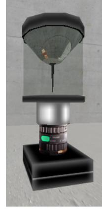
Figure 3.2: Unreal Static Mesh of Simulated Omnidirectional Camera
