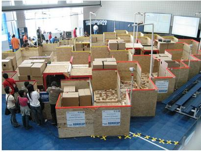
Figure 1.2: The RoboCup Atlanta 2007 NIST Reference Test Arena for Autonomous Mobile Robots
