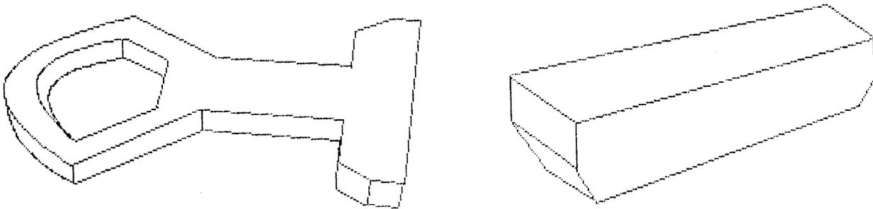
*figure 2.3a and b: 3D-model of a side plate and a spacing piece.*
