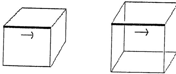
*figure 3a: an example of a (correct) hypothesis, the bold edges represent the two respective edges in the image (left) and the CAD-object (right) which will be checked in equivalence in topology and geometry.*
