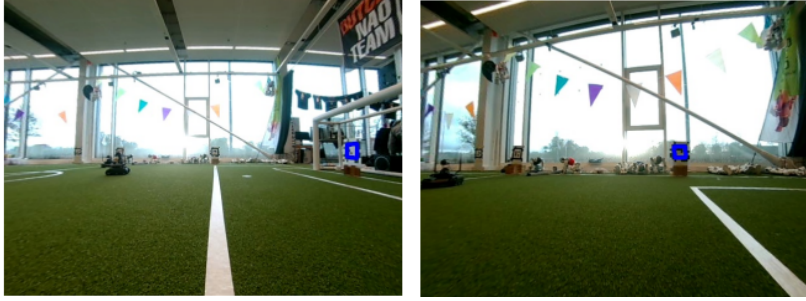
Fig. 9. Examples of marker detection around the field. In both images one tag is detected (blue square), while one marker to the left is not detected. Courtesy Dragomir et al.
