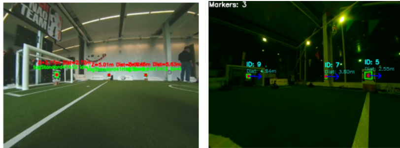
Fig. 10. Examples of successful marker detection at large distances and difficult lighting conditions. Courtesy Guarena Gonzalez et al.
