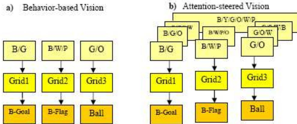
Figure 3: Behavior-based versus attention-steered vision: a) architecture of Behavior-based Vision [4]; different color-tables for different objects; b) architecture of Attention-steered Vision; multiple color-tables for each behaviors; B = Blue, Y = Yellow, G = Green, O = orange, W = White, P = Pink.
