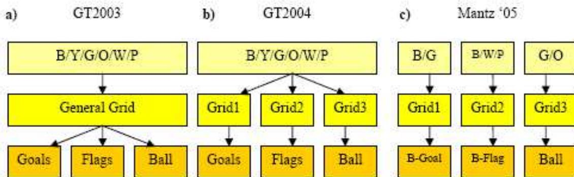
Figure 2: Generic versus object-specific steps in the object-recognition phase: a) architecture of the German Team 2003, only the shape evaluation (bottom) is object-specific; b) architecture of the German Team 2004, different scan-lines grids for different objects; c) architecture of Mantz [4]; different color-tables for different objects; B = Blue, Y = Yellow, G = Green, O = orange, W = White, P = Pink.
