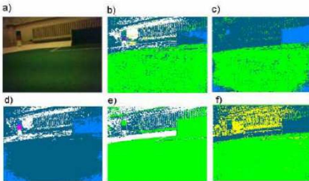
Figure 1: a) camera image (from [4]); b) segmented with the general color-table; c) segmented with the blue/green color-table for the detection of the blue goal; d) segmented with the blue/white/pink color-table for the detection of the blue flag; e) segmented with the green/white color-table for the detection of the field lines; f) segmented with the yellow/green color-table for the detection of the yellow goal.
