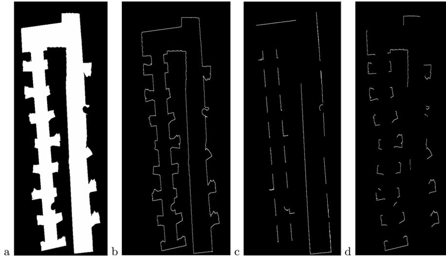
**Fig. 3.** The safe region of Fig. 2 ( $90^\circ$  degrees rotated). From left to right respectively a) The surface. b) The contour. c) The part of the contour which is an obstacle (wall). d) The part of the contour which is free (frontier).
