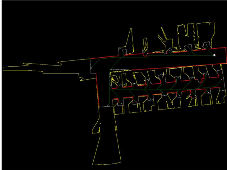
**Fig. 4.** The interpreted map of Fig. 2. The yellow contours indicate the observation regions. The grey contours indicate the exploration frontiers. The large white circle indicates the current position of the robot. The small white circles indicates potential observation points. The green line indicates a possible path to those observation points. Red lines indicate the walls.
