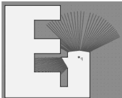
**Fig. 1.** The potential information gain of a candidate observation point  $q$  is the area  $A(q)$  that may be visible through the two free edges; this area is estimated by casting rays from  $q$ . Courtesy from [18].
