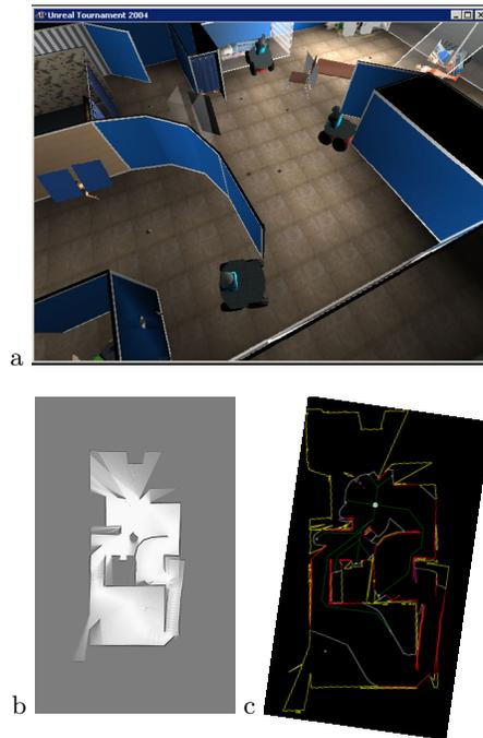
**Fig. 6.** Results of the Yellow-Arena map. Fig. b and c show the results of exploring a loop starting and ending in the curved wall in the center of the figures. On this map 9 observation points are found (one false positive).
