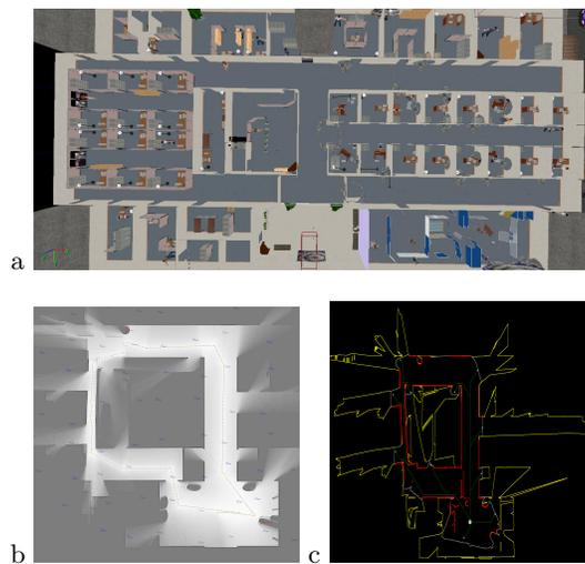
**Fig. 5.** Overview of the indoor area used for the 2006 RoboCup Virtual League Competition. Fig. b and c show the results of exploring a loop starting and ending in the large lobby at the bottom of Fig. a. On this map 11 of the 13 observation points are found.
