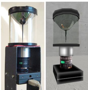
Figure 1: The catadioptric omnidirectional camera, real and simulated.
