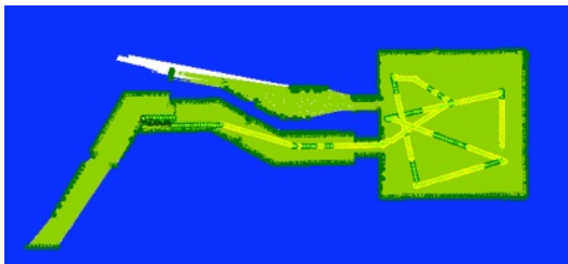
Fig. 6: Known traversability saved along the path of the robot.
