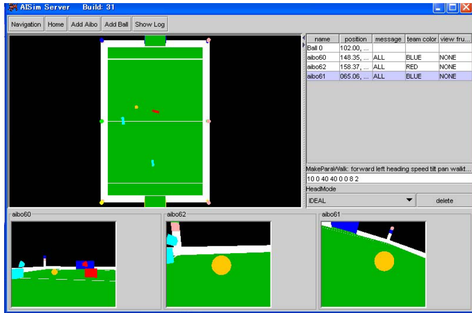
Fig. 5. The Simulator Server
