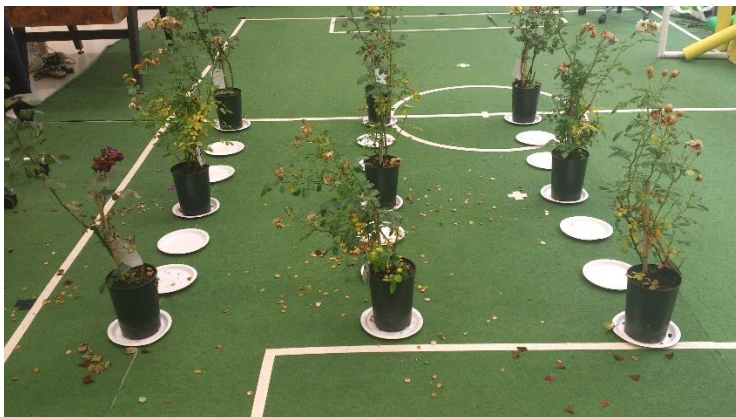
Figure 2: Rose Field, each white plate represents a node which the YouBot is not allowed to go to.
