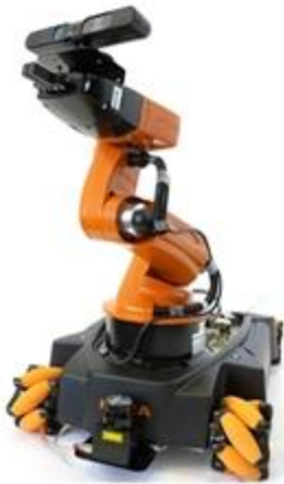
Figure 1: Kuka youBot equipped with Asus Xtion Pro Live camera, Xsens MTi-G-700 sensor and Hokuyo LX30 laserscanner
