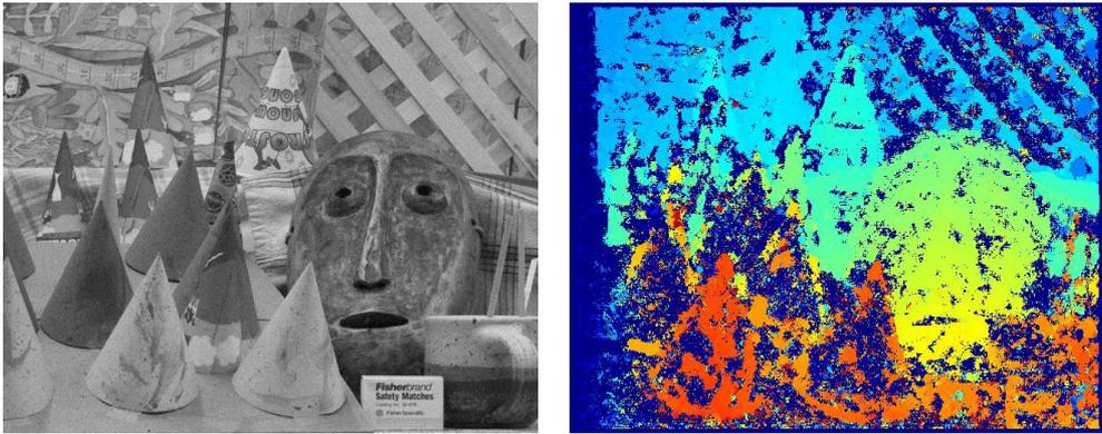
Figure 4.6: Original with noise (left), Unfiltered disparity estimate (right).
