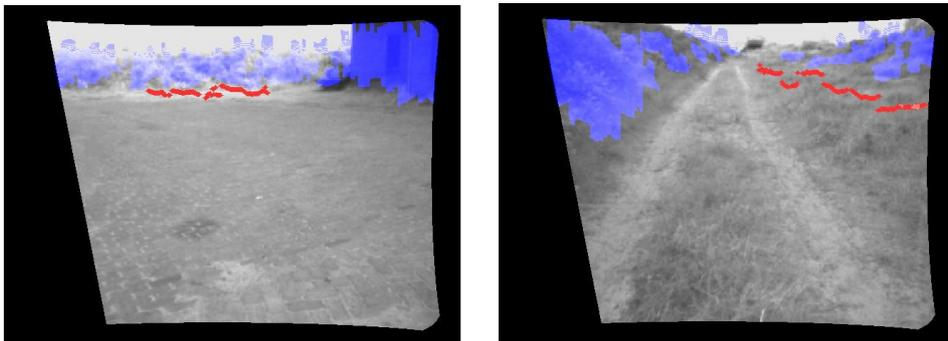
*Figure 4.19: Problem of parameter choice. Using a step height of 0.45 meter and a hysteresis threshold of [2.0 3.0] we can detect the negative obstacle (left). However, false detections can appear e.g. on top of grass polls (right).*
