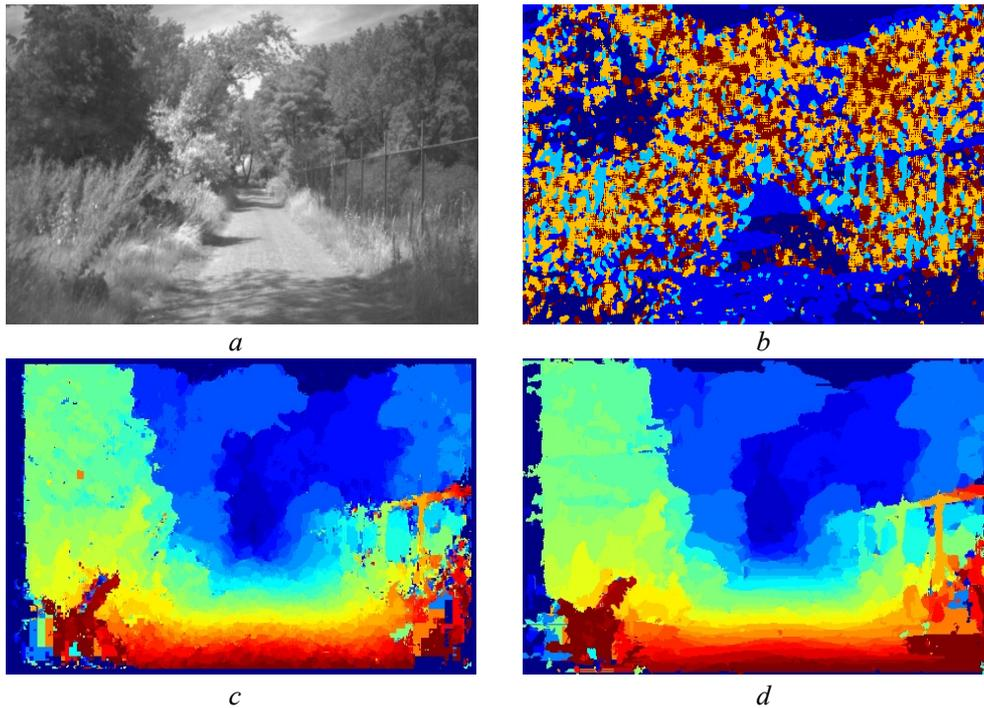
Figure 6.1: Using texture segmentation to improve disparity estimate. Left image of stereo image pair (a) and its texture segmentation (b), disparity map (c), texture enhanced disparity map (d).
