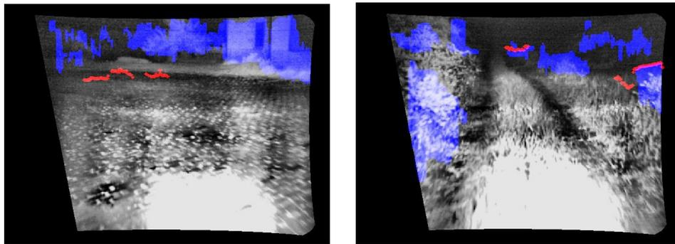
*Figure 4.21: Problem of parameter choice. Using a step height of 0.45 meter and a hysteresis threshold of [2.0 3.0] we can detect the negative obstacle (left). However, false detections can appear e.g. on top of grass polls (right).*
