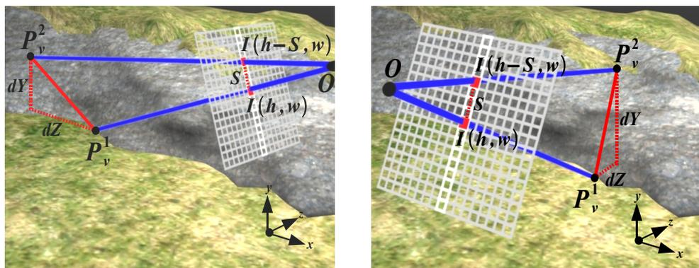
Figure 2.19: Influence of viewing angle on estimated slope. Estimated slope is less than true slope(left), Estimated slope is equal to the true slope (right).
