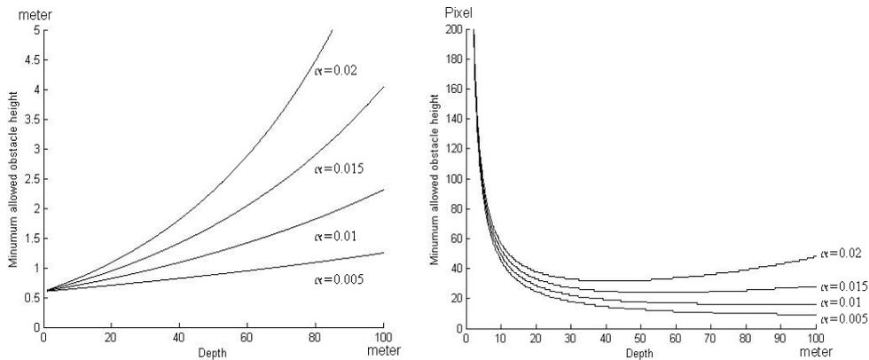
Figure 3.8: Depth dependent height threshold in meters (left) and pixels (right).
