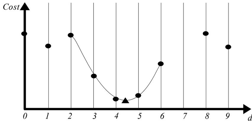
Figure 2.17: Sub-pixel accuracy (triangle), pixel accuracy  $d = 4$ .
