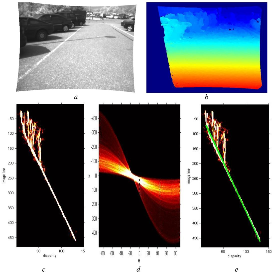
Figure 2.24: Original image (a), Disparity map(b), V-Disparity map(c), Hough transform(d), V-Disparity with extracted ground plane (green) using Hough transform(e).
