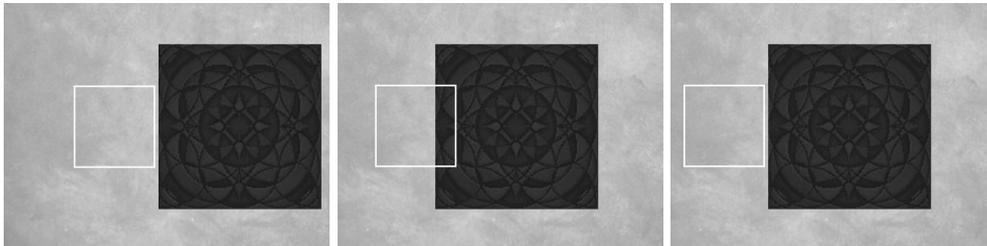
*Figure 2.10: Reference window (left) Correct matching window (middle) Chosen matching window (right).*
