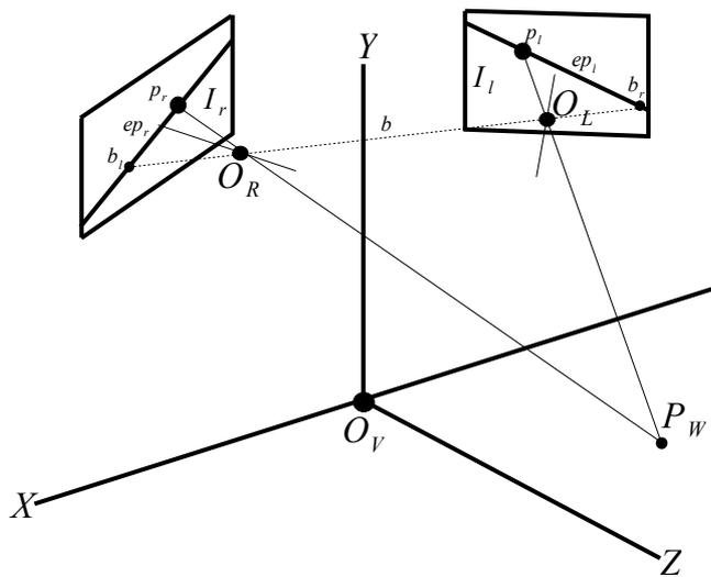
Figure 2.5: Non rectified binocular camera system.
