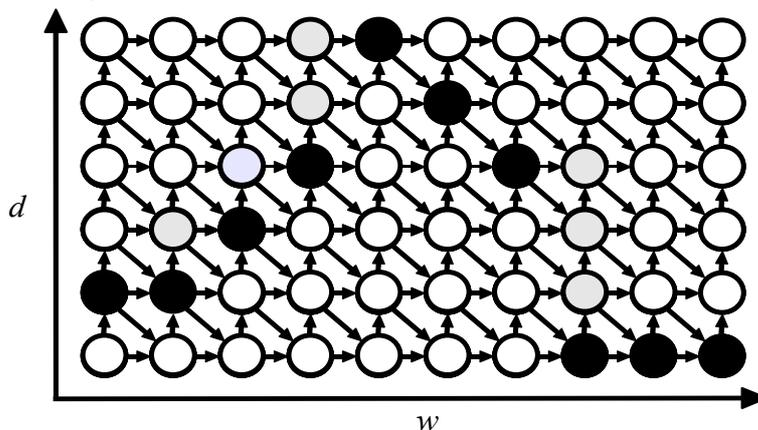
Figure 2.14: DSI based MRF with disparity path (grey and black nodes).
