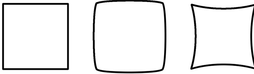
Figure 2.3: Effects of radial distortion, undistorted (left), barrel distortion (middle), pincushion distortion(right).
