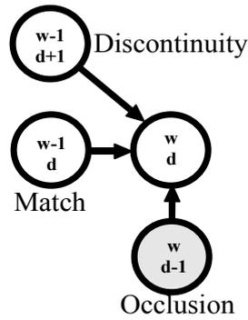
Figure 2.15: Allowed relations between MRF nodes.
