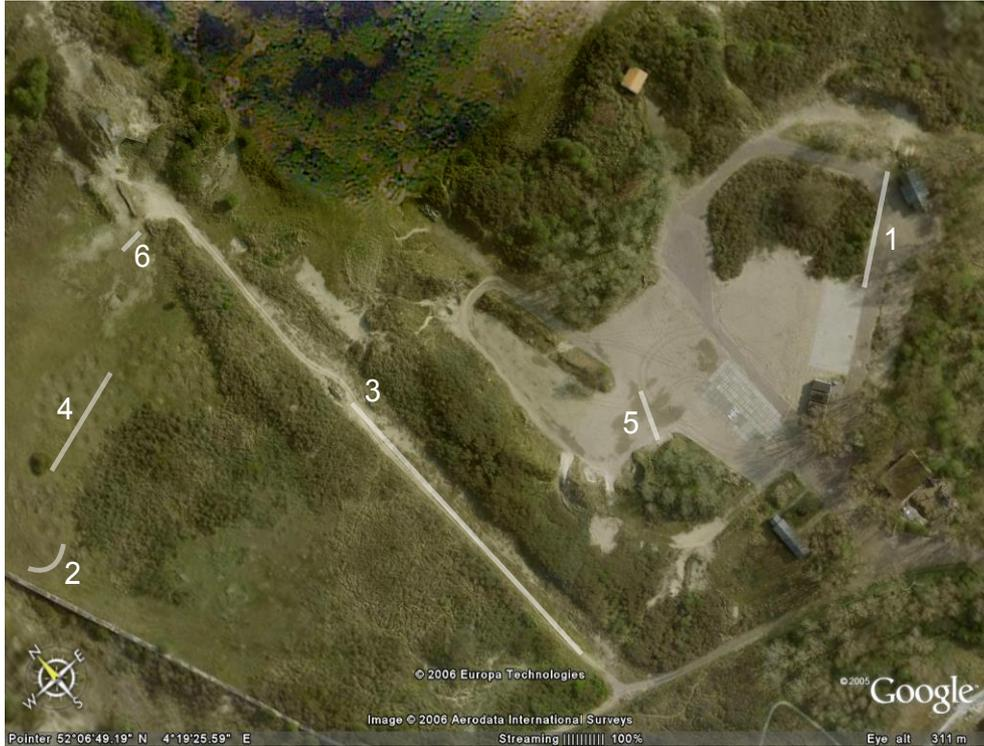
Figure 3.10: Test terrain, 1 big gap 2 concrete wall, 3 Rock pile, 4 Holes, 5 Sand plane, 6 Trunks.
