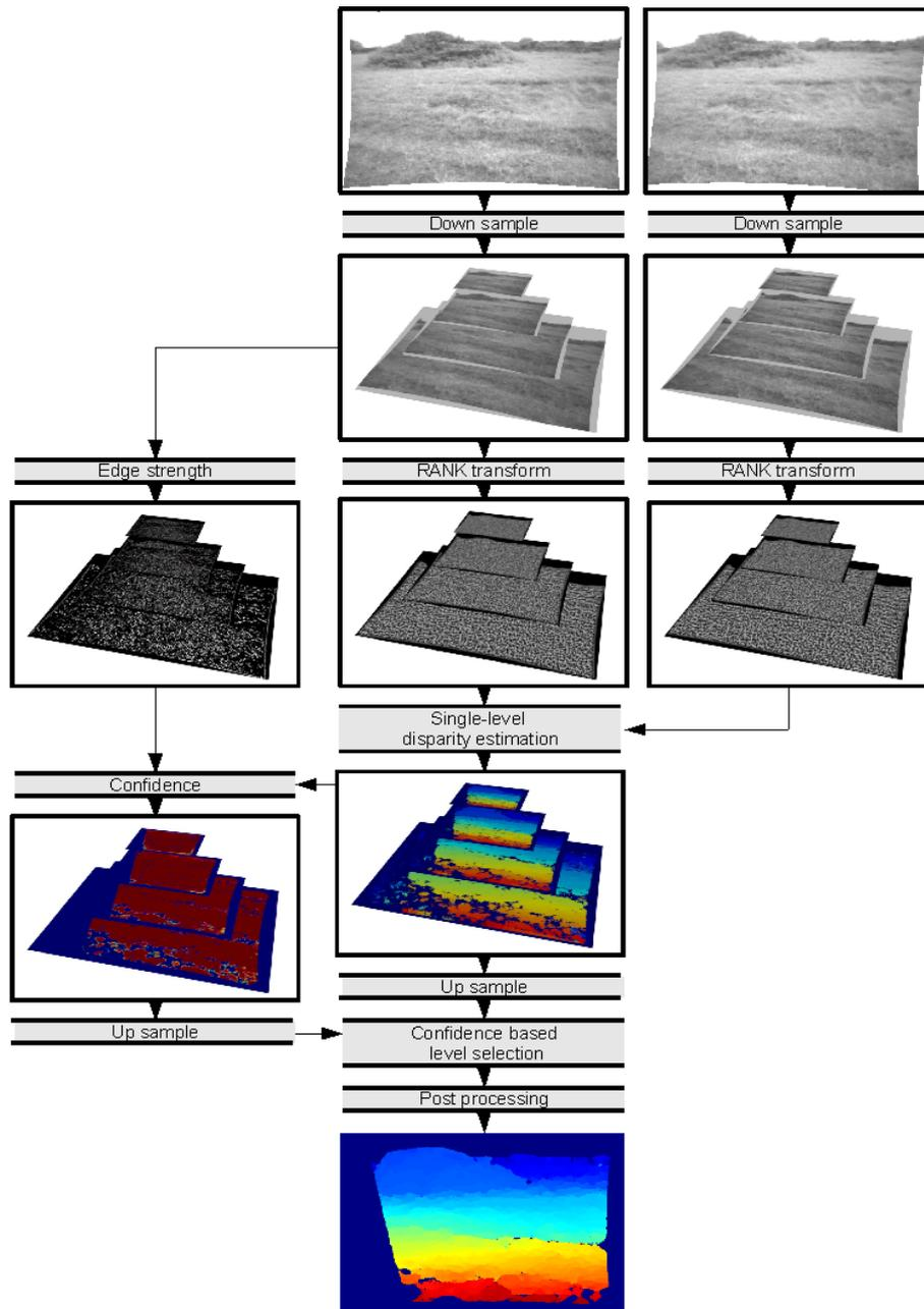
Figure 3.2: Steps in our disparity estimation algorithm.
