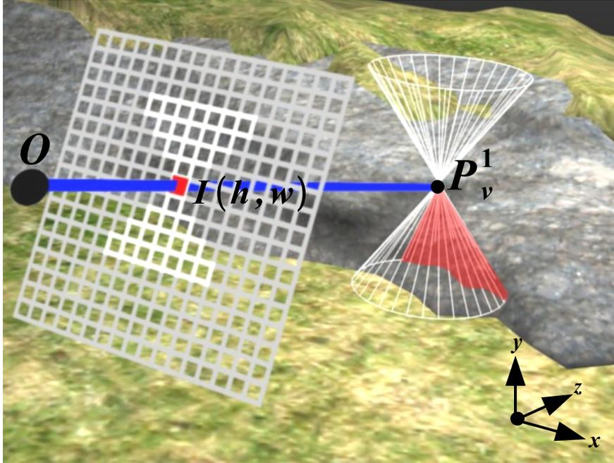
Figure 2.23: Truncated cones approach. Truncated cones are projected to two triangles in the image. red terrain is compatible with  $P_v^1$ .
