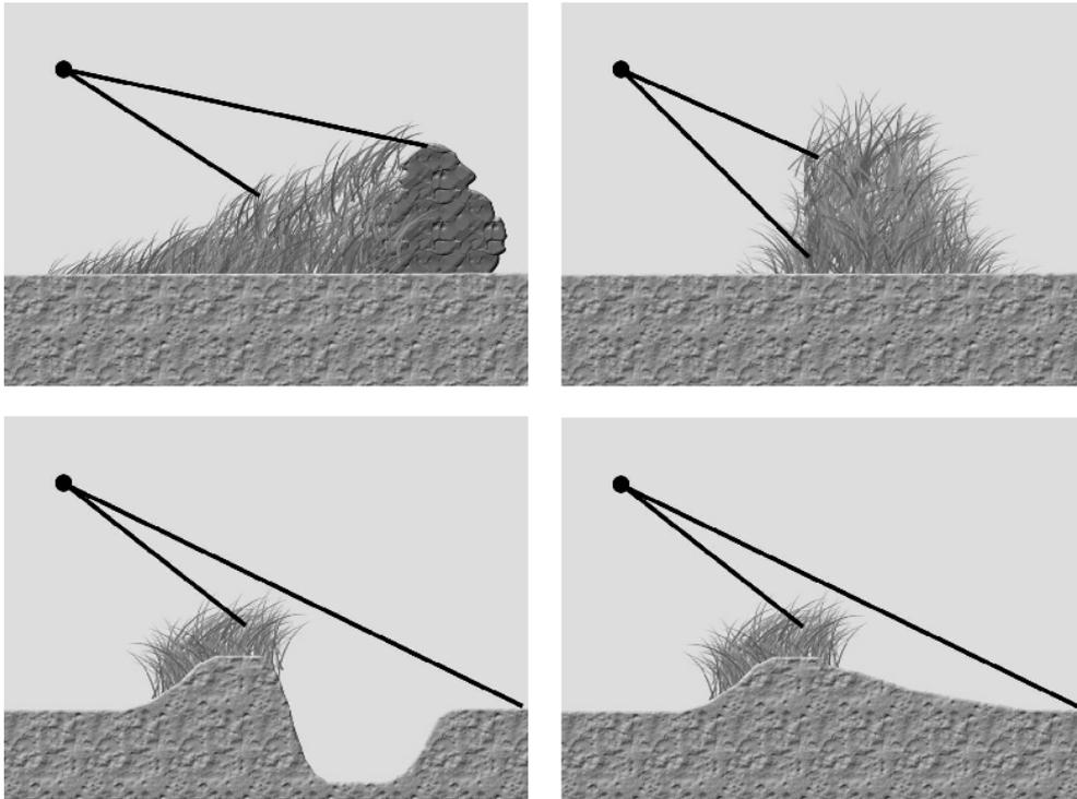
*Figure 2.25: Limitations of stereo based OD.*
