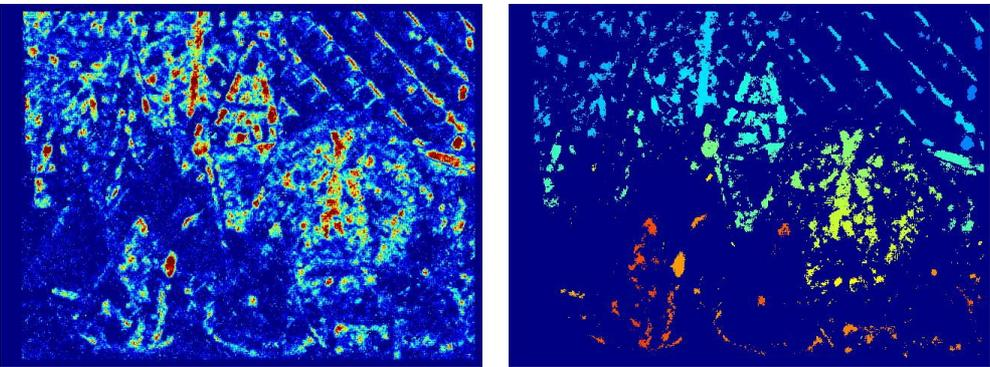
Figure 4.8: Winner Margin third best (left), Filtered disparity map at 70% error reduction (right).
