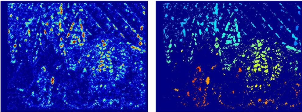
Figure 4.9: Winner Margin second best (left), Filtered disparity map at 70% error reduction (right).
