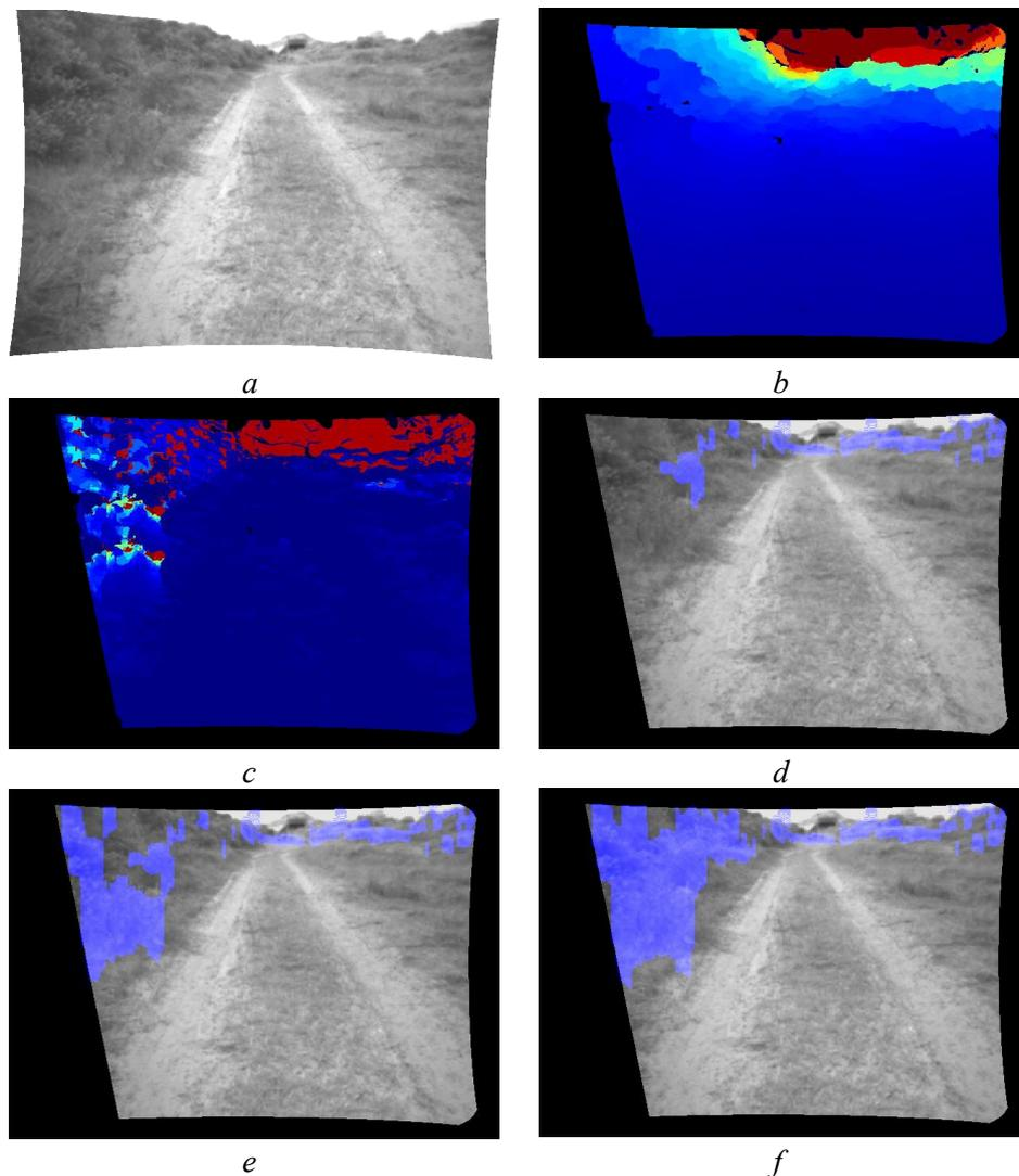
Figure 4.14: Original image (a), computed depth map (b), computed slope map(c), Regular threshold 0.75 (d), hysteresis thresholding [0.5 0.75] (e) and [0.25 0.75] (f).
