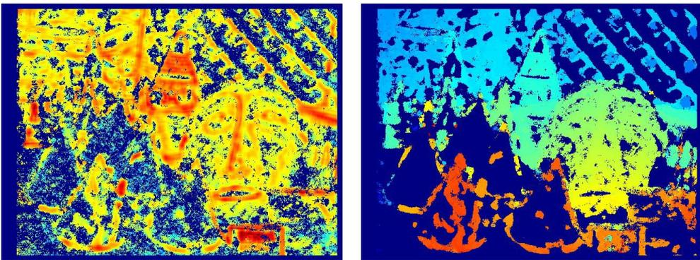
Figure 4.7: Novel validity measure (left), Filtered disparity map at 70% error reduction (right).
