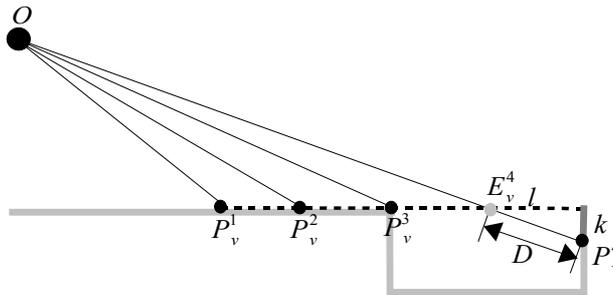
Figure 2.22: Negative obstacle detection.
