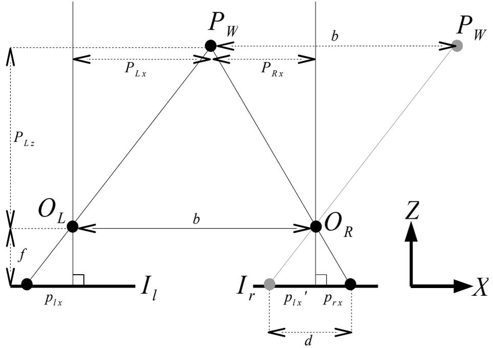
Figure 2.6: Stereo geometry.
