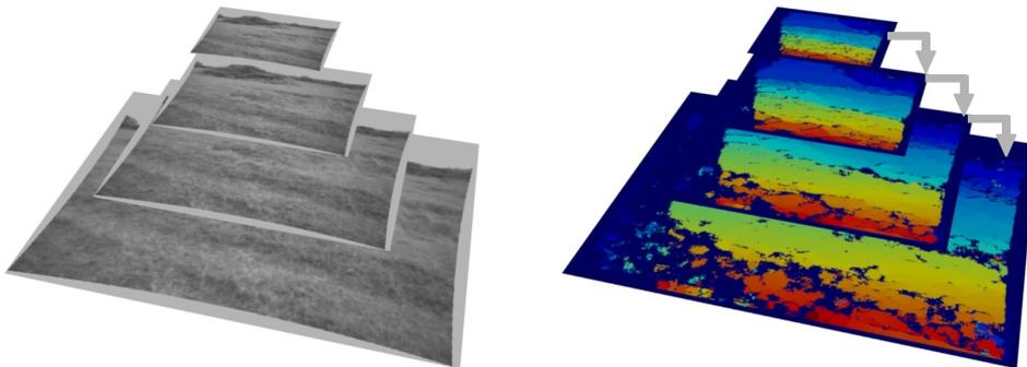
*Figure 2.13: Multi-resolution disparity estimation.*
