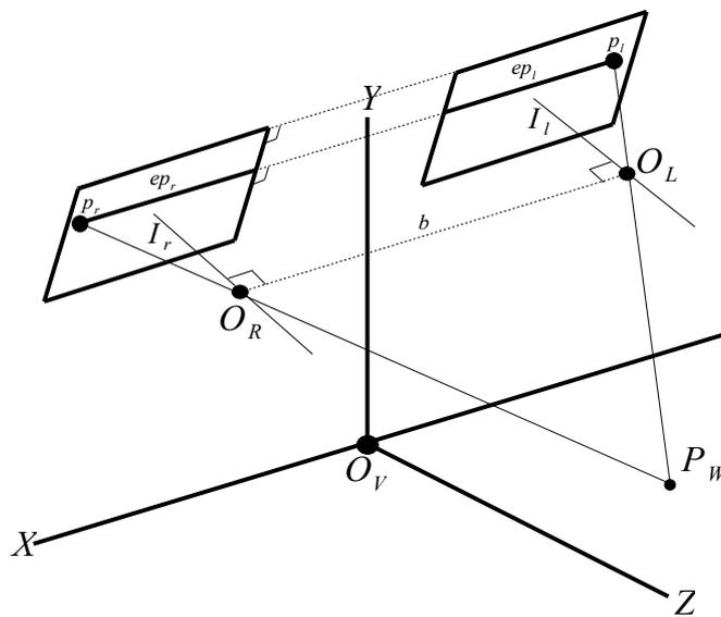
Figure 2.4: Photo parallel binocular camera system.
