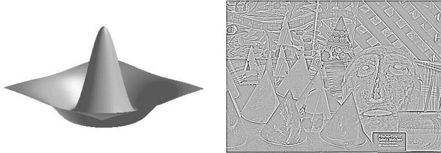
Figure 2.9: LoG kernel (left), LoG filtered image (right), original image figure 2.11.
