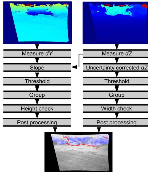
Figure 3.3: Obstacle detection system overview, positive obstacles left column, negative obstacles right column.
