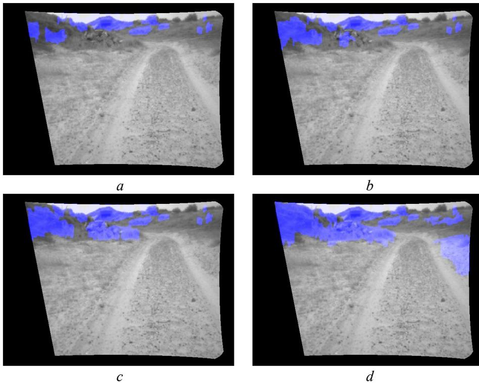
Figure 4.13: Effect of hysteresis thresholding, 0.75-0.75(a) 0.75-0.25(b) 0.75-0.15(c) 0.75-0.05(d).
