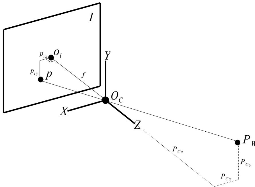
Figure 2.2: Pin-hole camera model.
