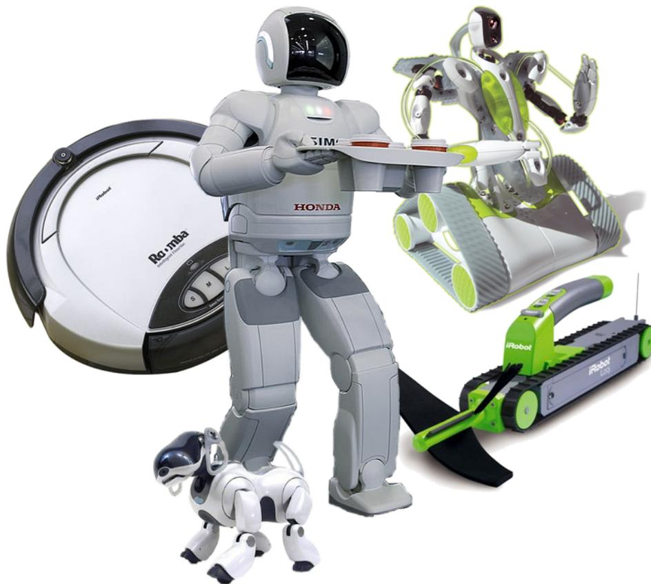
Figure 1.1: Several robots developed for the consumer market. From the top left, going clockwise: iRobot Roomba vacuum cleaner, Honda ASIMO humanoid robot, Meccano Spykee spy robot, iRobot Looj gutter cleaning robot and Sony AIBO entertainment robot.
